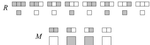
Figure 1: Rules and mappings. Shaded cells represent value 1.  $R$  shows how the "name" of an ECA rule is derived: each of the 8 possible ECA initial state is shown in bigendian order; below it, the next state of the central cell is shown; the rule is "named" by reading off the values of the next state. Here,  $R$  is the transition table for ECA rule 150 (10010110<sub>2</sub>).  $M$  represents the coarse grain mapping 0110, with grain  $g = 2$ .
