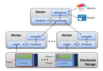
Figure 4: The architecture for distributed recurrent cohort analysis queries
