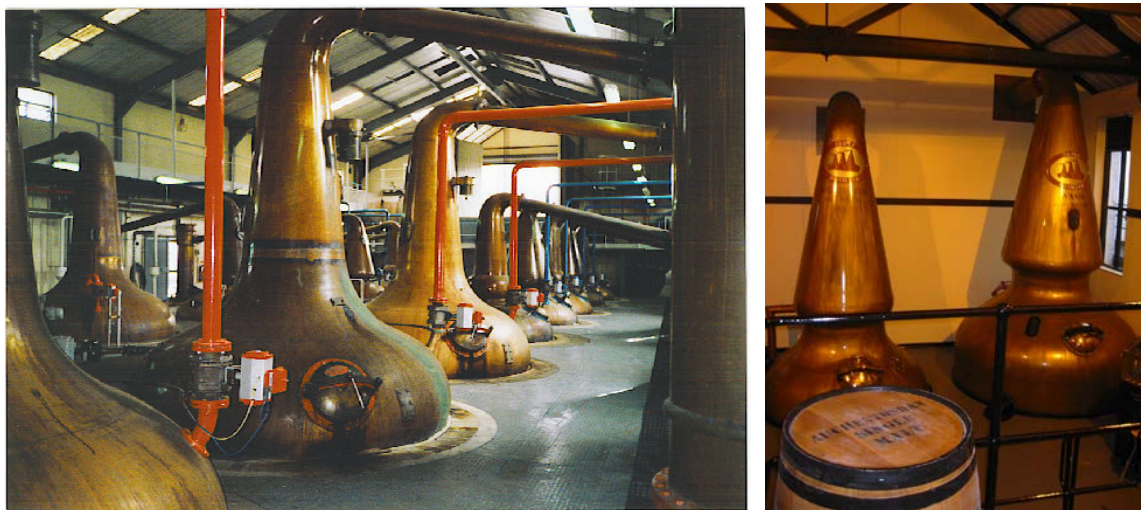
Figure 7. Left : Swan necked copper stills in the Glenfiddich distillery. Right : Copper pot stills at Auchentoshan Distillery in Scotland.
