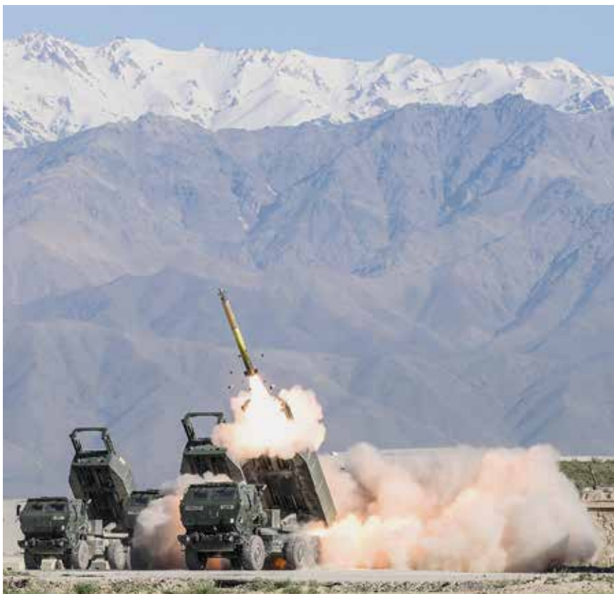
A Guided Multiple Launch Rocket is fired from a M142 High Mobility Artillery Rocket System launcher.
