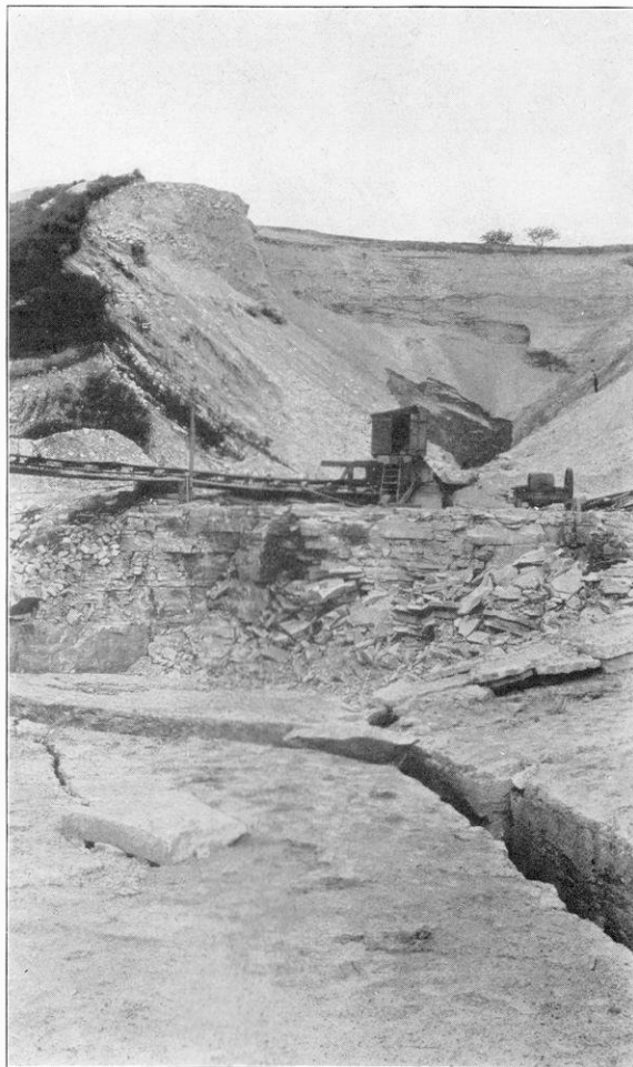
Waukesha Lime & Stone Co.'s quarry, at Waukesha. The limestone beds in the foreground belong to the dense, fine-grained, compact, even-bedded type of Niagara limestone. The bank of loose material in the back ground is a gravel deposit of glacial origin, made up largely of limestone pebbles.
