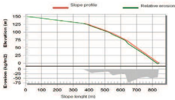
**Fig. 6.** The evolution of the erosion process on slope H29 (*Podzol*, maximum involvement of the soil particles at 648m - 74.2 kg/m<sup>2</sup>, the maximum deposit at 842m - 11.5 kg/m<sup>2</sup>)
