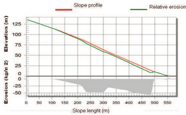
**Fig. 3.** The evolution of the erosion process on slope H2 (*Aluvisol*, maximum involvement of soil particles at 484m - 57.1 kg/m<sup>2</sup>, the maximum deposit at 556m - 6.72 kg/m<sup>2</sup>)
