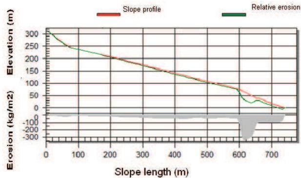
**Fig. 7.** The evolution of the erosion process on slope H6 (*Dystric Cambisol*, maximum involvement of the soil particles at 615m – 342kg/m<sup>2</sup>, the maximum deposit at 741m – 10,5 kg/m<sup>2</sup>)
