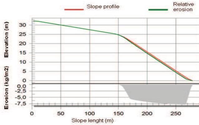
**Fig. 5** The evolution of the erosion process on slope H26 (*Prepodzol*, maximum involvement of the soil particles at 264m - 7.79 kg/m<sup>2</sup>, without deposit)
