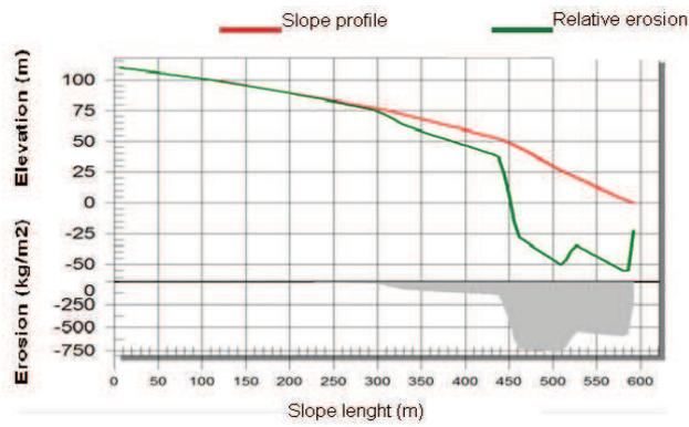
**Fig. 4.** The evolution of the erosion process on slope H8 (*Histosol*, maximum involvement of soil particles at 509m - 767kg/m<sup>2</sup>, without deposit)
