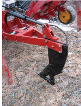
Fig 2. One of the three soil penetrating cones.
