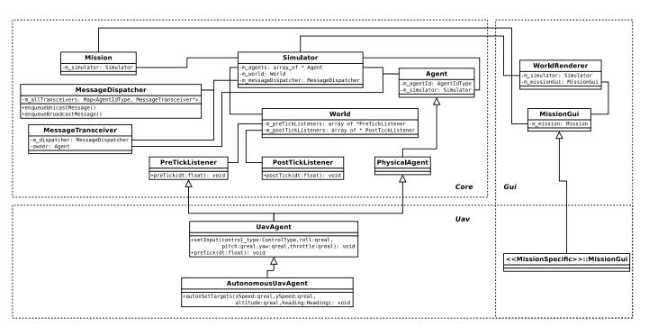
Fig. 1. Simplified Class Diagram of the Simulator
