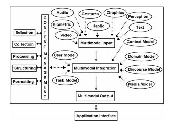
Fig.2. Logical diagram of the presentation generation process
