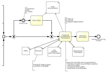
Figure 1. Section of a process model of the role Maintenance Manager
