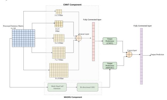
The authors propose an ensemble framework **ECMAG** (illustrated in Fig 3) which consists of 2 components – Convolutional Neural Network for Texts (CNNT) and Multi-Head Attention pipelined to Bi-GRU (MHGRU). The details of the components are elucidated in the following sections.
