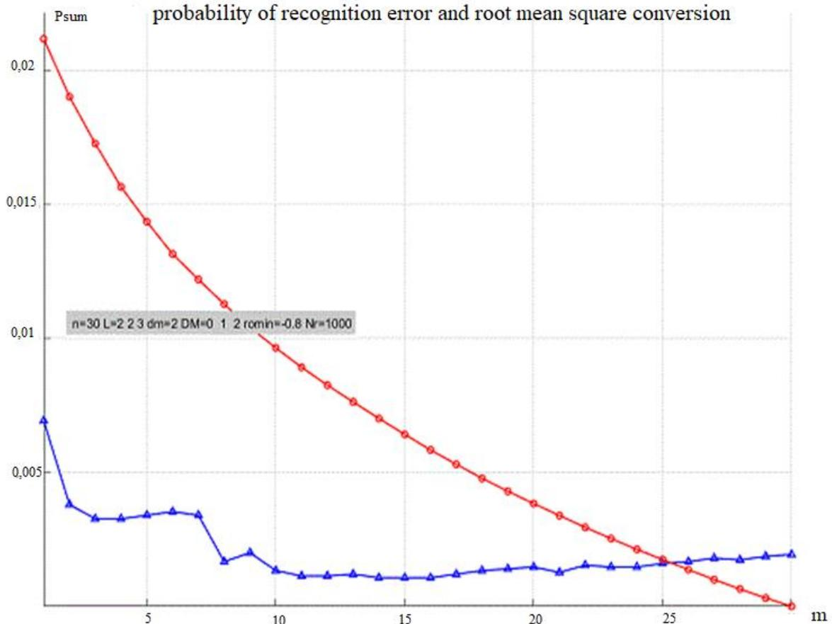
**Figure 4:** Dependences for the total probability of error and UPC transformation on the dimension of the feature vector after the transformation algorithm of the principal components
