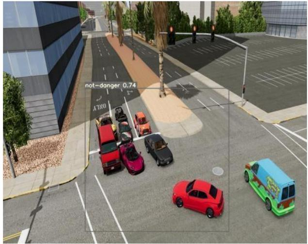
Figure 15: Inference result of Yolov7 [28]
