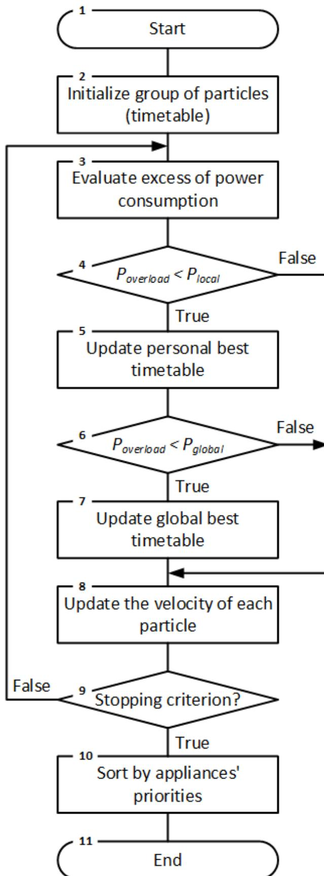
**Figure 2:** Particle swarm optimization algorithm with priority system
