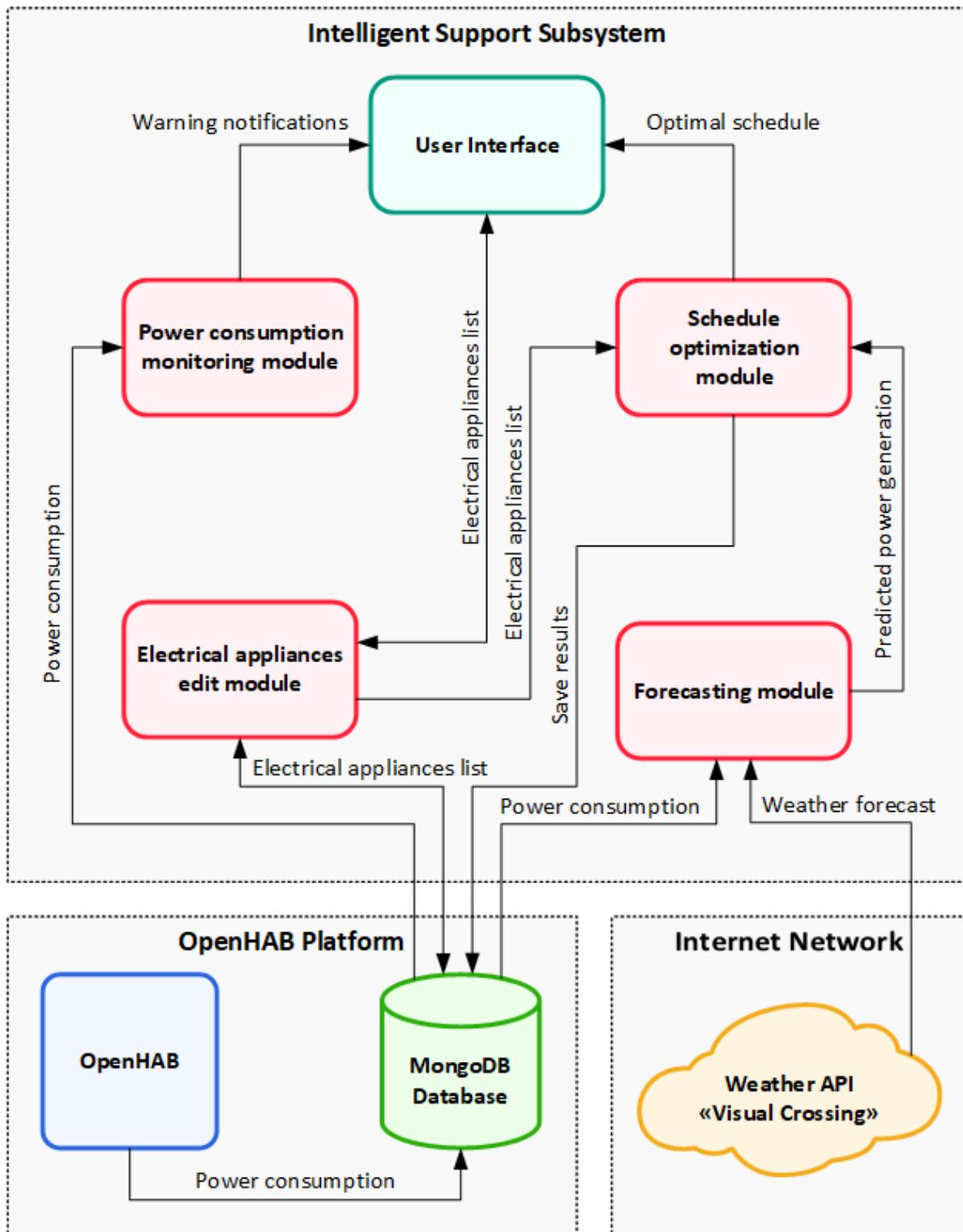
Figure 3: Structural/functional diagram of the developed subsystem
