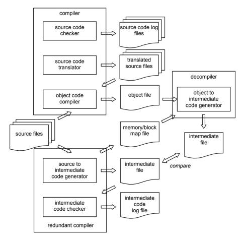
Fig. 4. Code compilation using diverse software
