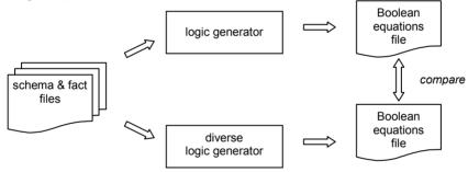
Fig. 3. Logic generation using diverse software
