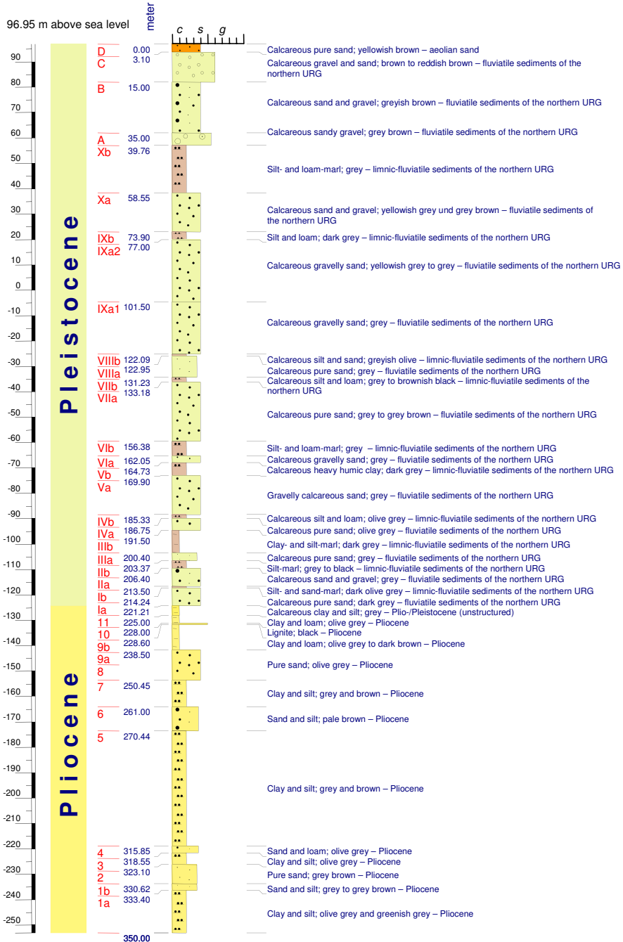
Fig. 3: Schematic geological section of the Viernheim research borehole showing a summary of the sedimentological units.
