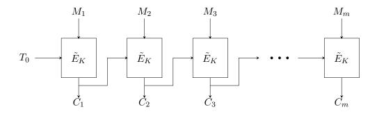
Fig. 1. TBC mode of operation
