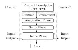
Figure 5: Architecture and Workflow of TASTY
