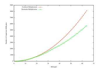
Figure 8: Size of Multiplication Circuits
