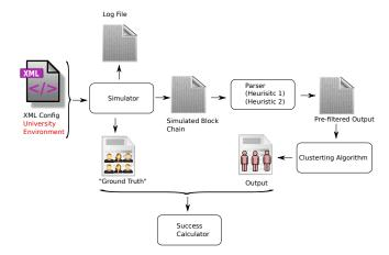
**Fig. 1.** Experimental setup used throughout our simulations. The outputs of our Bitcoin simulator are pre-filtered according to Heuristics I and II and then fed as input to our clustering algorithm. The clustering result is then compared with the "ground truth" that is emulated by our simulator.
