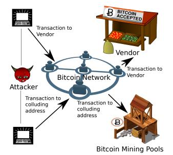
Figure 3: Sketch of a double-spending attack against fast payments in Bitcoin. In typical cases, the attacker  $\mathcal{A}$  dispatches two transactions that use the same BTCs in the Bitcoin network. The double-spending attack is deemed successful if the BTCs that  $\mathcal{A}$  used to pay for  $\mathcal{V}$  cannot be redeemed (i.e., when the second transaction is included in the upcoming Bitcoin block).
