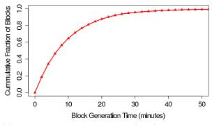
(a) Block generation times in Bitcoin. Assuming a (time) bin size of 2 minutes, the block generation function can be fitted to a shifted geometric distribution with p = 0.19. Refer to Appendix A for further details.
