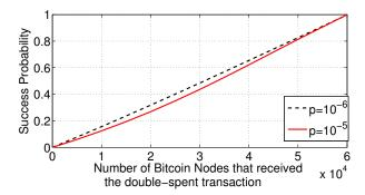
**Figure 5:** P<sub>S</sub> for various values of  $\eta_{\mathcal{A}}^k$  and  $\eta_{\mathcal{V}}^k$ , with  $p = 10^{-6}$ ,  $\delta t = 10$  seconds,  $t_0 = 0$ ,  $t_s = \delta t$  and the number of peers in the network is 60000. Further details can be found in Appendix B.
