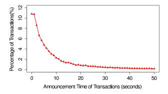
Figure 11: Distribution of time intervals between announcements of successive transactions. To measure the transaction announcement times, we parsed the block chain of Bitcoin and we counted the number of transactions in each block. To generate the plot, we assumed that transactions are announced uniformly at random within two successive block generations.
