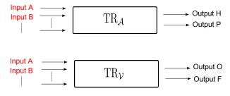
Figure 2: Example construction of  $TR_{\mathcal{A}}$  and  $TR_{\mathcal{V}}$ . Here, we show two different transactions with the same inputs and different outputs.  $TR_{\mathcal{A}}$  and  $TR_{\mathcal{V}}$  can share a subset of their inputs—in which case  $\mathcal{A}$  only tries to double-spend a subset of the BTCs that she pays with.
