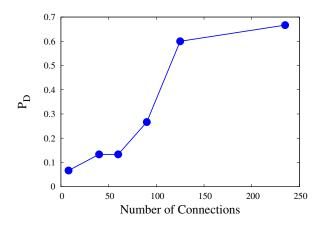
Figure 10: The connectivity of  $\mathcal{V}$  as a security parameter. We measure  $P_D$  with respect to the number of connections of  $\mathcal{V}$ . Here, we consider a setting where  $\mathcal{V}$  is located in Asia Pacific,  $\Delta t = 3.0$  seconds and  $\mathcal{A}$  controls 4 helpers. As the number of connections of  $\mathcal{V}$  increases, the probability that  $\mathcal{V}$  receives both  $TR_{\mathcal{A}}$  and  $TR_{\mathcal{V}}$  also increases.
