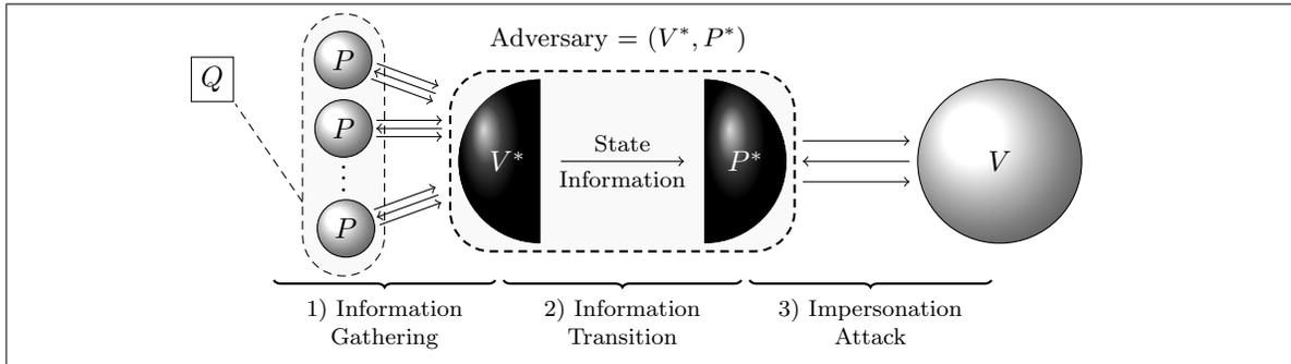
Figure 1: The smart-card authentication model.
