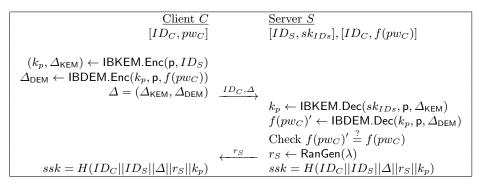
Fig. 2. Generic construction for IBPAKE
