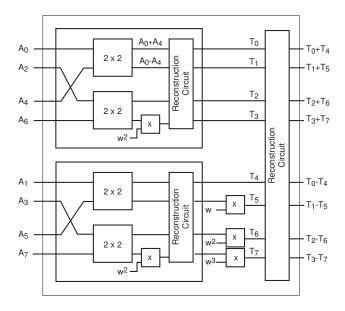
**Fig. 1.** Construction of the  $8 \times 8$  NTT circuit iteratively.
