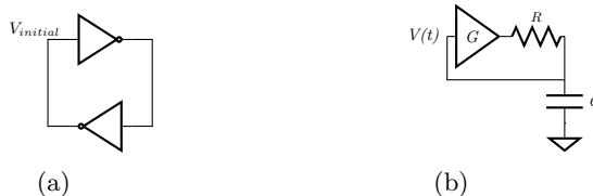
Fig. 1: (a) The logical circuit of an SRAM cell. (b) The small signal model of bistable element in metastability
