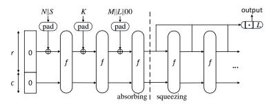
Figure 3: KMAC processing one message block
