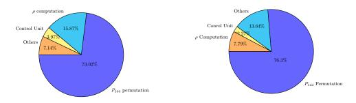
Figure 6: Distribution of Components by #Slices (left) and #LUTs (right)
