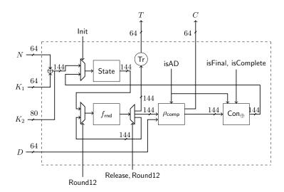
Figure 3: Hardware circuit diagram for Beetle[Light+]
