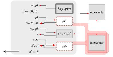
Figure 4: The IND-CPA game after expanding the key generation algorithm's definition and inlining the query-recording hash oracle. The red boxes represent the inline operator.
