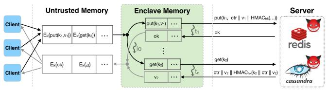
Fig. 5: Proxy architecture for concurrent query processing.
