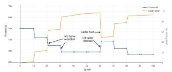
Fig. 4: Threshold tuning during a run of YCSB-C
