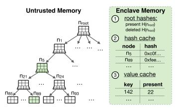
Fig. 3: Caches optimize reads of MB-tree's state.
