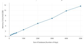
Fig. 9: Proxy memory usage by number of keys.
