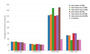
Fig. 11: Throughput with various cache sizes, using 1 thread, RocksDB server, and 5 million keys.
