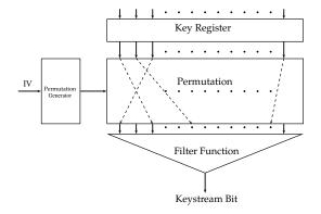
Figure 14: The FLIP stream cipher
