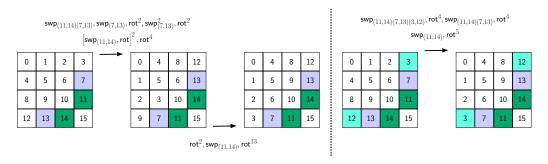
Figure 9: Transposition  $\tau$  can also be done in 128 (resp. 64) cycles with 2 (resp. 3) swap operations.
