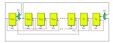
Figure 15: 2nd Circuit for Knuth Shuffle
