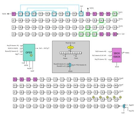
Figure 12: Combined ENC+DEC PRESENT circuit using only 6 swaps with no permutation latency
