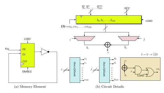
Figure 16: 3rd Circuit for FLIP
