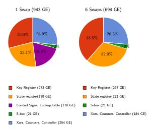
Figure 17: Breakdown of the area requirements of the individual components of PRESENT in the 1 and 2 swap architectures
