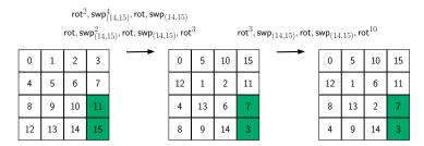
Figure 10: Performing  $\sigma$  with  $swp_{(11,15)}$  and rot in 2 full rounds, i.e  $2 \times 64$  cycles.
