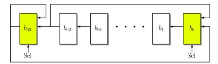
Figure 1: Shift register circuit with (subsequent) 2 scan flip-flops
