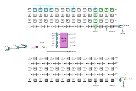
Figure 11: PRESENT circuit using 6 swaps (12 scan flip-flops)
