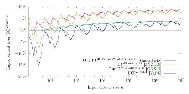
Figure 9: Improvement in size in percentage of our 2/4 hybrid, the 4-way UCs of [Val76, ZYZL19] over Valiant's 2-way UC for  $15 \le n \le 10^7$  with logarithmic x axis. We note that the different graphs are in the same order as in the legend.
