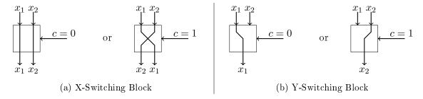
Figure 2: Programmable switching blocks [KS08a].
