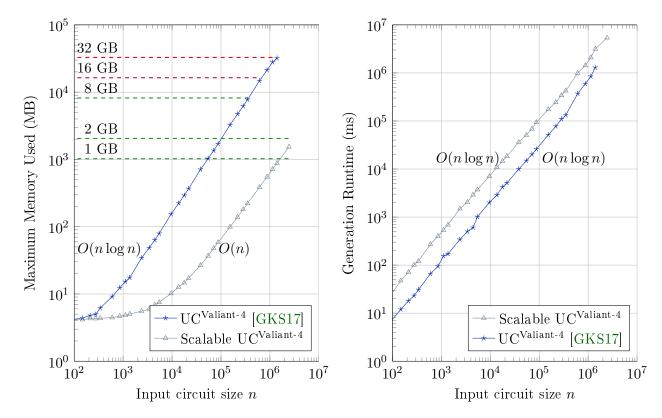
Figure 13: Comparison of the maximum memory used between our per-block and [GKS17]'s UC generation. [GKS17]'s implementation runs out of 32 GB of memory for n > 1398100 nodes.
