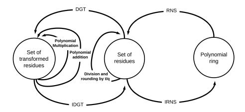
Fig. 1. An optimized state machine for the cyclotomic polynomial arithmetic. Data is kept in RNS' domain and encapsulated by DGT for polynomial multiplications and additions, similar to *double*-CRT, but solely on RNS for division and rounding by t/q.
