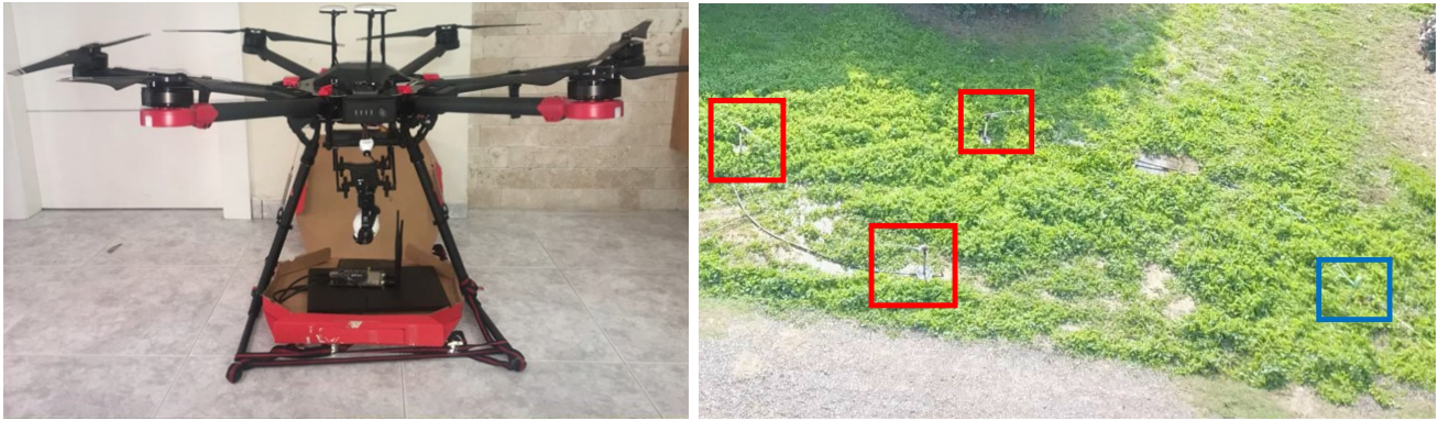
Fig. 12: Left: The drone carries a laptop and SDR that are used to trick cellular GreenIQ. Right: Sprinklers (boxed in red) are operated by cellular GreenIQ (boxed in blue) as a result of a cloud server impersonation attack that was conducted from a drone.
