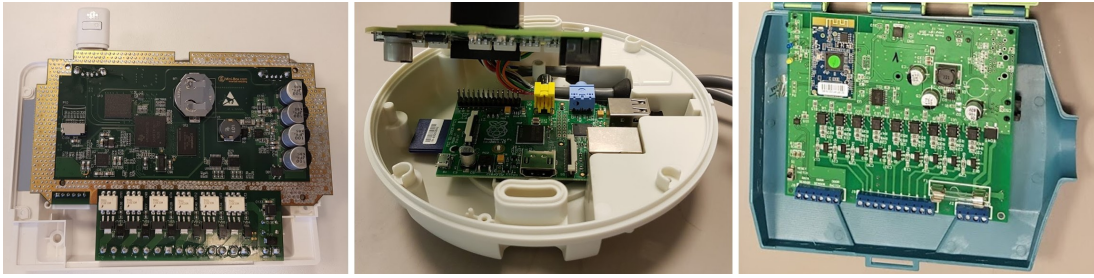
Fig. 3: SoC board of RainMachine (left), GreenIQ (middle), and BlueSpray (right).
