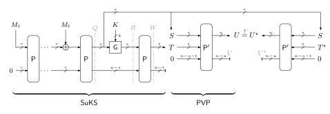
Fig. 3: The SuKS-then-PVP construction StP. The message M is first injectively padded into r-bit blocks  $M_1 \dots M_\ell$ .
