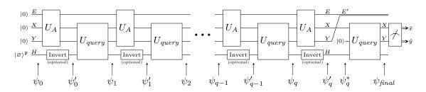
Figure 4: Circuit describing the two-sided zero search game. We drew an Invert before/after every query. Only a subset of these will actually be contained in the circuit.  $\hat{p}$  is the probability that  $(\hat{x}, \hat{y})$  is bad.
