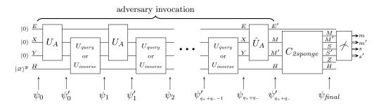
Figure 7: Circuit used in the collision-resistance proof for the sponge construction.
