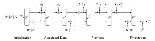
Figure 1: Ascon's mode of operation (encryption phase)
