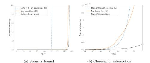
Fig. 3: Comparison of the state-of-the-art security bound, new security bound, and best known attack for the Ascon-Hash mode with parameters (b, c, r, r', n) = (320, 256, 64, 64, 256).
