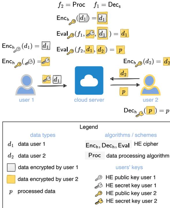
Fig. 14. HPRE for homomorphic evaluation of multi-user data.
