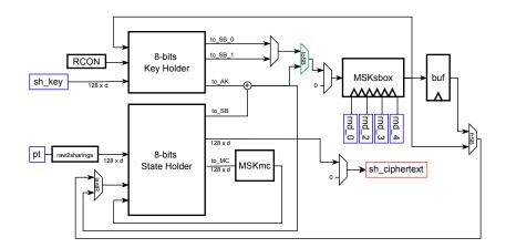
Fig. 3. Global Architecture of the 8-bit serial implementation.
