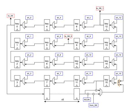
Fig. 5. 8-bit implementation: architecture of the key holder.
