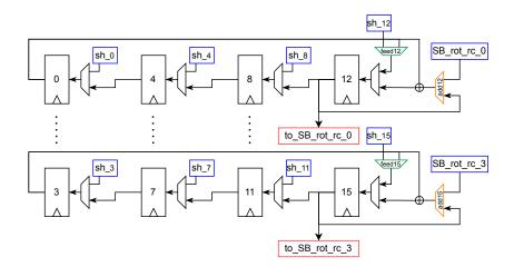
Fig. 8. 32-bit implementation: architecture of the key holder.
