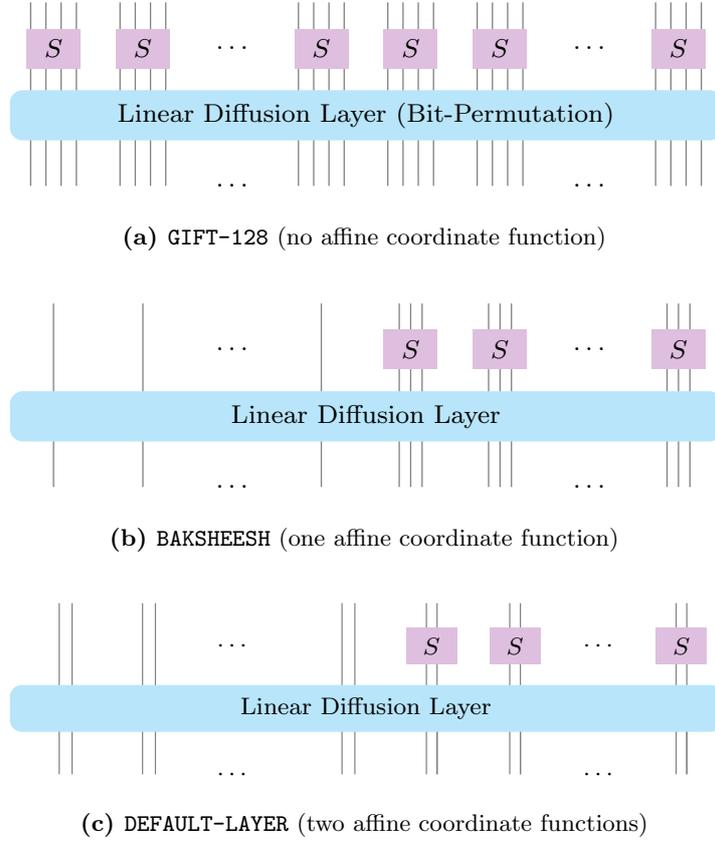
**Figure 2:** Equivalent schematic for one round (showing partial non-linear layer)
