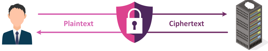
Fig. 1. Secure Outsourcing with HE: The client encrypts sensitive data and then transmits the ciphertext over a network to the remote cloud server. The cloud server can then execute an algorithm over the ciphertexts and generate an encrypted answer, which is transmitted back to the client. Lastly, the client can decrypt and receive the result of the computation. No information about the inputs or outputs is revealed to the cloud.
