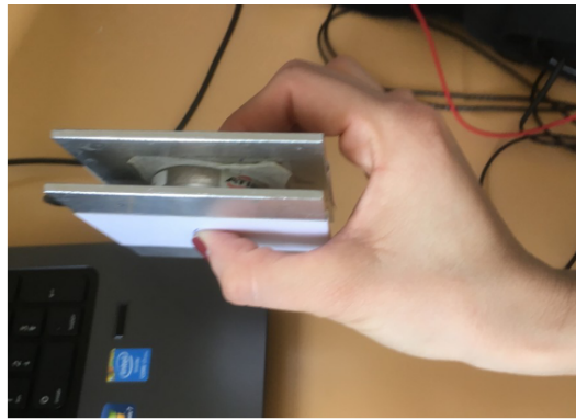
FIGURE 4.1: Held between fingers, the grip-force sensor (strain gage) measures small variations of pressure which can arise from motor simulation when watching an action or hearing action verbs
