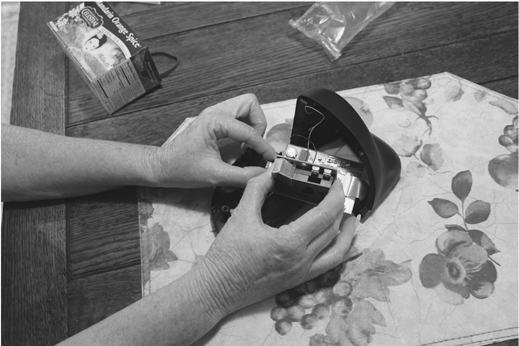
Figure 2.17. Setting up Specks for monitoring particulate matter at participants' monitoring locations. Photographs by Citizen Sense.
