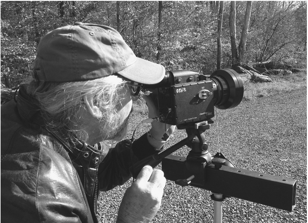
Figure 2.2. Frank Finan monitoring emissions at a compressor station using a FLIR camera. Photographs by Citizen Sense.
