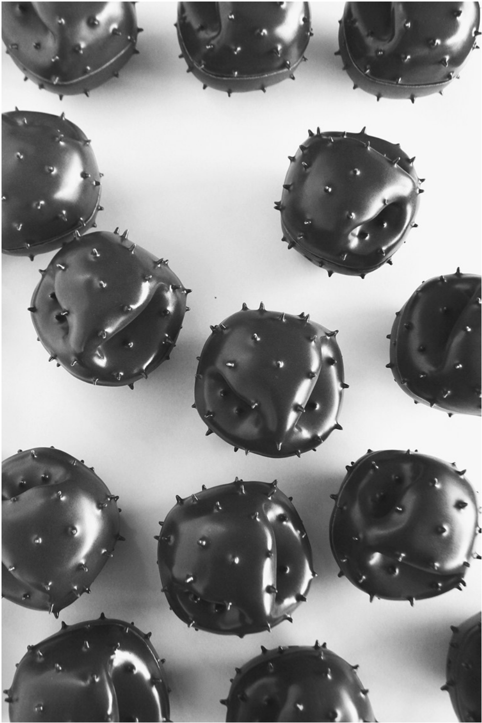
Dustboxes, a particulate-matter sensor for monitoring air quality developed by Citizen Sense. Photograph by Citizen Sense.
