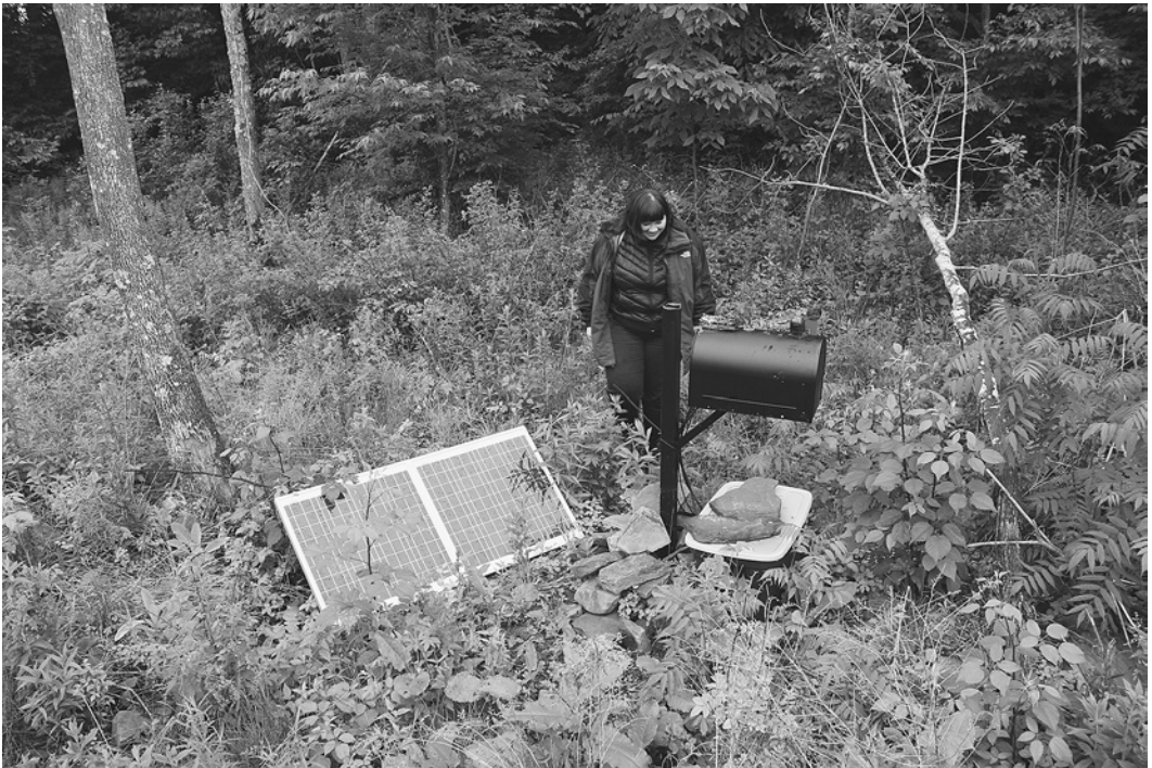
Figure 2.20. Frackbox installations through winter 2014 and summer 2015 at compressor station. Photographs by Citizen Sense.
