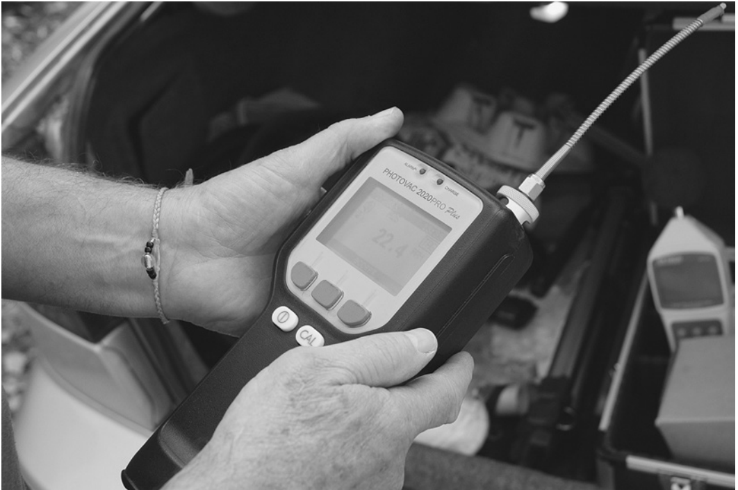
Figure 2.9. Frank Finan showing different devices for measuring VOCs, including a Global Community Monitor bucket for collecting air samples, and a handheld VOC monitor. Photographs by Citizen Sense.
