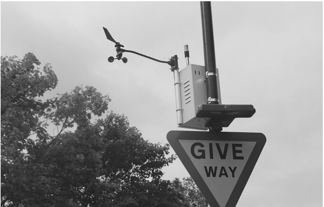
Figure 3.9. Air-pollution monitoring infrastructure sensing wind speed and direction with air pollutants in Deptford to document possible emissions from the Thames Tideway Super Sewer construction. Photograph by Citizen Sense.
