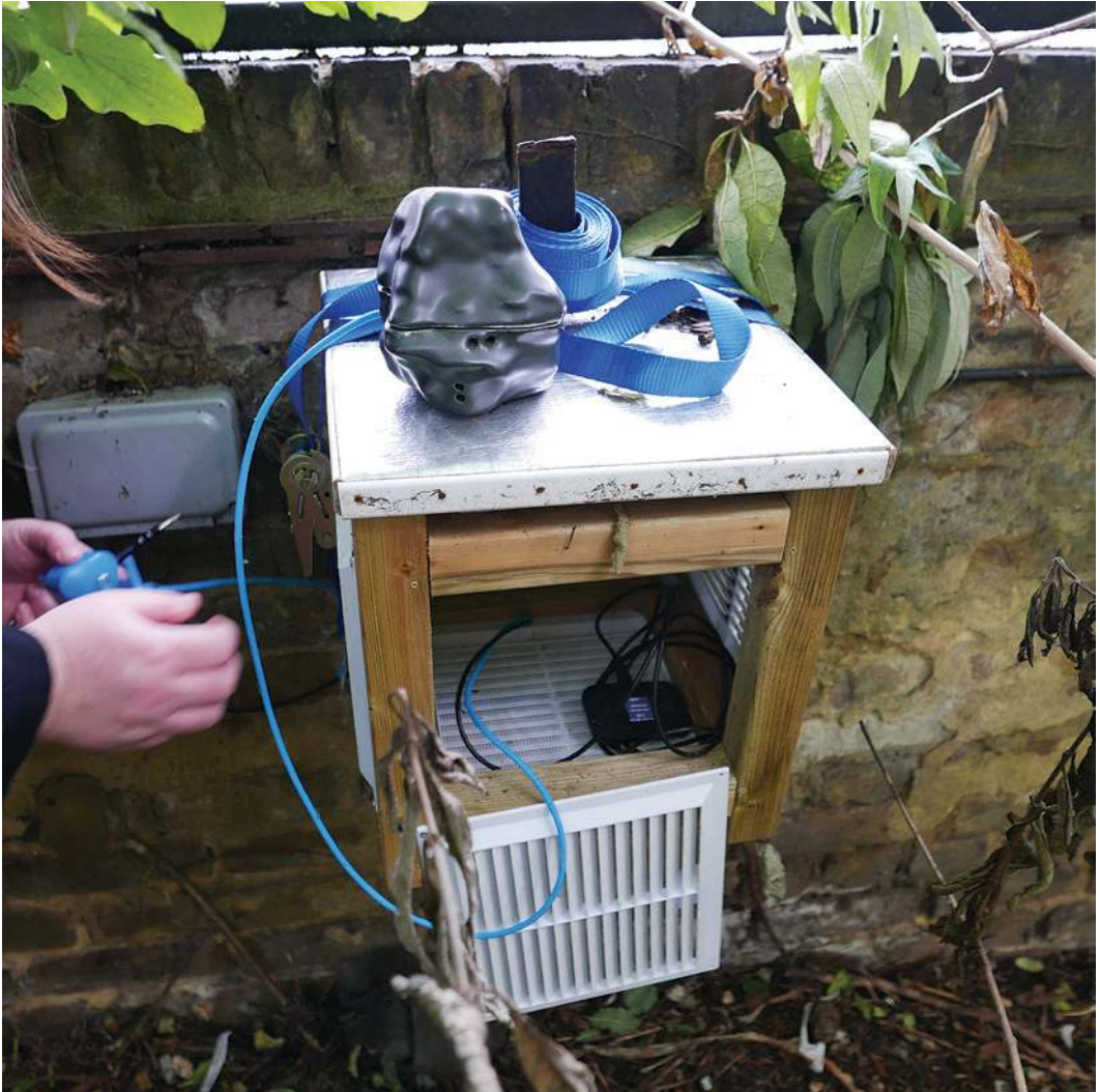
Plate 4. Installation of Dustbox in the Beech Street regulatory air-quality monitor. This monitor, sited at the edge of a traffic tunnel and near the Barbican Tube Station, regularly registers high levels of nitrogen oxides and particulate matter. Photograph by Citizen Sense.
