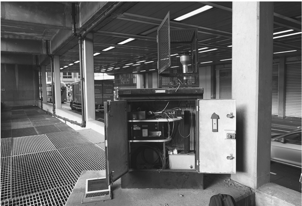
Figure 4.7. Installation of Dustboxes in the Beech Street regulatory air-quality monitor. This monitor, sited at the edge of the Beech Street tunnel and near the Barbican Tube Station, regularly registers high levels of nitrogen oxides and particulate matter. Photographs by Citizen Sense.
