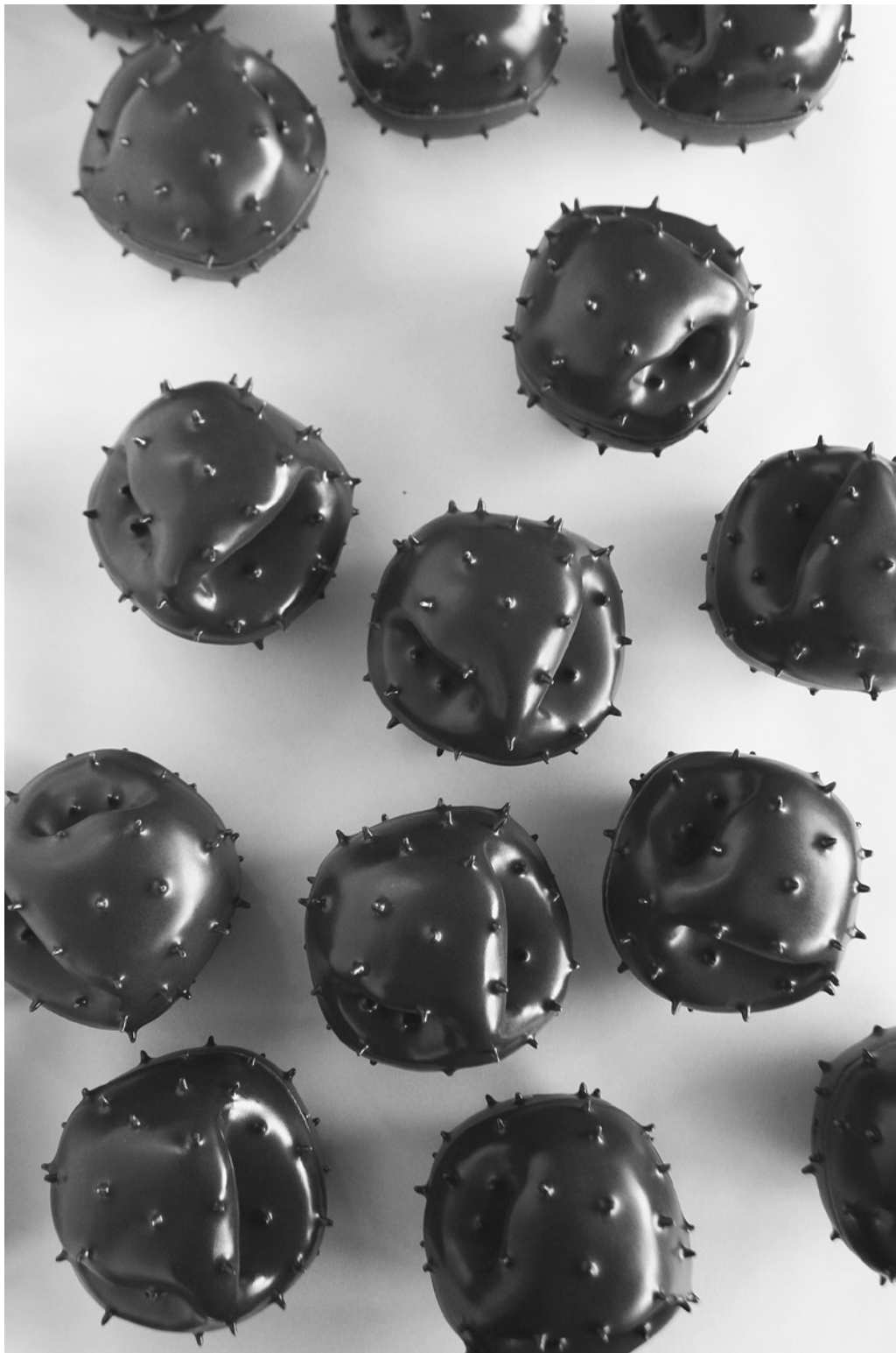
Figure C.2. Dustboxes, a particulate-matter sensor for monitoring air quality developed by Citizen Sense. Photograph by Citizen Sense.
