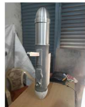
Towfish for inspection of underwater pipeline
