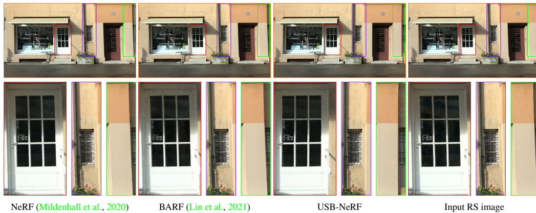
Figure 11: Qualitative comparisons on real-world datasets captured by GoPro HERO6. The images are captured on a moving tram in constant direction. It demonstrates that even both NeRF and BARF can render clear images, the recovered scene is distorted. Our method can correctly un-distort it.
