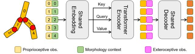
Figure 1. The framework of *MetaMorph* (Gupta et al., 2022). On this two-leg robot for example, its nodes are ordered by depth-first tree search, with the torso node as the tree root. *MetaMorph* concatenates proprioceptive observations and morphology context as node inputs, processes them with a shared embedding layer, a transformer encoder and a shared decoder sequentially. Exteroceptive observations are concatenated as decoder inputs if needed.
